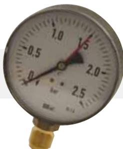
Manometer 1/2" 0-2,5 bar/25 m VS, Ø100 mm
