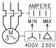
**LAYOUT (A)****Calibration of thermal cut-out 8)(A)p. 3**
