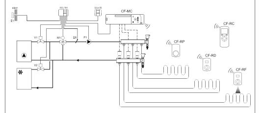
The valves V1 and V2 are for on/off actuators (TWA, ABV or AMZ 112 also available with switch for activating boiler or heat pump etc.) for supplying either heating (V1) or cooling (V2) to the mixing circuit (M1, S3 and P1). M1 could also be a 2-way valve in the return on the primary side.
