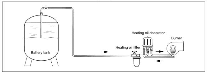
Installation of the heating oil deaerator above the oil level, e.g. underground tank
