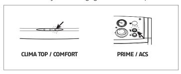
If a "LOCKOUT SHUTDOWN" occurs, wait about 30 seconds before resetting the burner.
