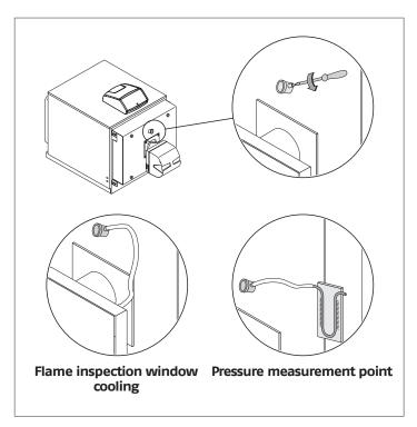
A rubber socket is attached to the flame inspection window. If this is used as a pressure measurement point, leave the screw in place in order to close off the pressure measurement line during normal boiler functioning. If the rubber socket is used to cool the flame inspection window, remove the screw to ensure an adequate air flow.
