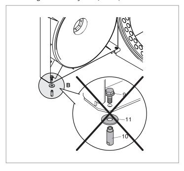
The first time you open the door, remove the spare hinge assembly 'B' [bushing (10), bolt (9), and washer (11)] opposite the hinged side of the door.
