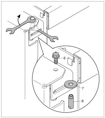
fit the bushing (8), bolt (6) and washer (7) to the opposite side of the door.
