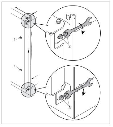
Make sure that the door is properly adjusted after every maintenance operation.
