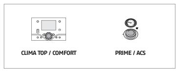
adjust the timer thermostat/s or temperature controller to the desired temperature (~20°C);
