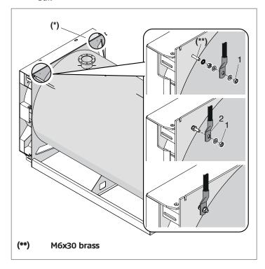
Another hole (\*) in the left side of the boiler head can also be used to earth the appliance. If you wish to use this hole for the earth connection, remove the terminal fittings from the right of the head and move them to the left earthing point.
