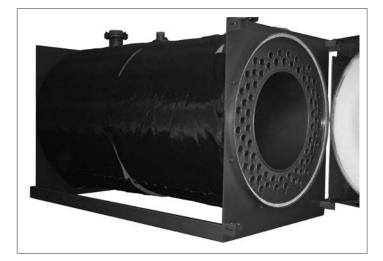
Fit the fixing clips on the turbulators and push the turbulators into the flue gas pipes until the clips make contact.  $\frac{1}{2} \int_{-\infty}^{\infty} \frac{1}{2} \int_{-\infty}^{\infty} \frac{1}{$
