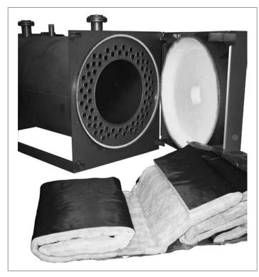
Fit the insulation over the rear of the combustion chamber first, wrapping it around as shown in the figure.
