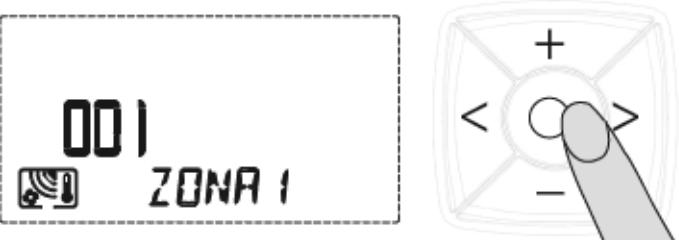
The unit affiliation process is over; now it is possible to remove the cable from the unit and insert it in a new unit to be affiliated. When the affiliation processes are over, completely remove the cable from the control panel.
